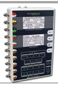
The SECULIFE PS300 is an easy-to-use patient simulator in which all parameters can be selected through a graphic display. Autosequences for BDM and printing can be selected. 10 Patient connections are available. An extension to SpO2 function is possible. Two channels for blood pressure and 49 arrhythmias are available.
