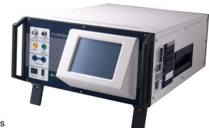
Using internal precision non-inductive test loads in the range of 0  $\Omega$  to 6400  $\Omega$  in a previously unavailable 1  $\Omega$  increment the SECU**LIFE** ESXTRA offers biomedical engineers, service engineers and manufacturers compatibility. Just in case, we have included the capability to add an external load, guaranteeing 100% test load requirement compatibility for years to come.
