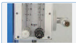
AIR O 2 / MIXER (PN 12432A70) It allows setting flow rate and percentage of O 2 by adjusting the inputs according to the corresponding table. It is possible to have an output with only Air, O 2 , or both and the other one with Vacuos.
