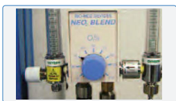
NEO2 Air/O 2 Blender (PN 12368A70) It allows having settable percentage O 2 on two outputs with different flow rates: 31/min or 151/min
